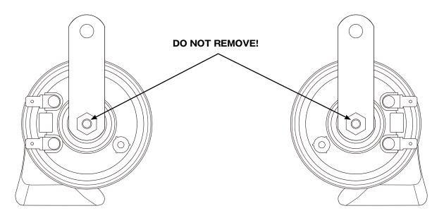
The nut can be loosened to rotate and adjust the bracket position.
